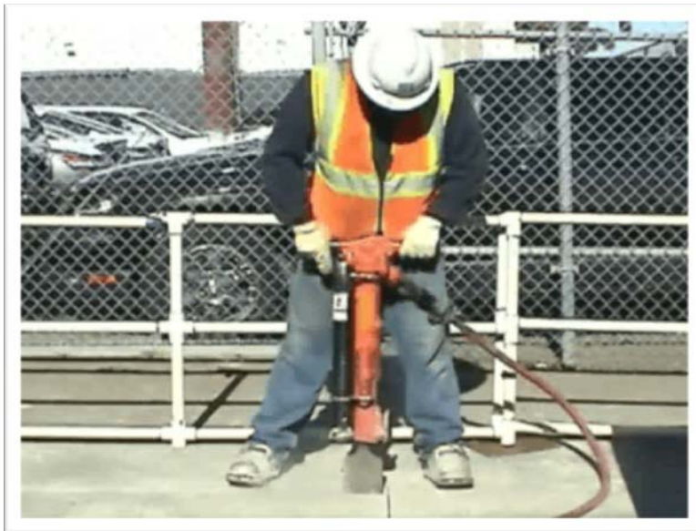
Figure 2: Worker using jackhammer with Lift Assist. (Note: Lift Assist is the black cylinder attached to the jackhammer)
