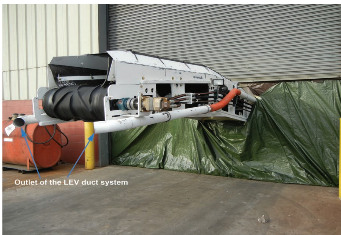
Figure A. Configuration for laboratory tracer gas test (Photo by NIOSH)
