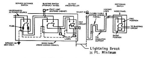
Recommended Installation of Shooting Station and Accessory Arrangement for Using Arcontroller b. A grounded switch shall be installed between the blasting switch and the power circuit at a distance not less than 15 ft (4.5 m) from the blasting switch.
