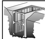
Additionally, excavated or other materials must be at least 2 feet back from the edge of a trench; and
