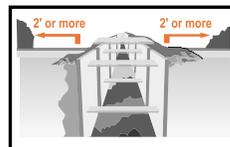
A safe means of egress shall be provided within 25 feet of workers in a trench.
