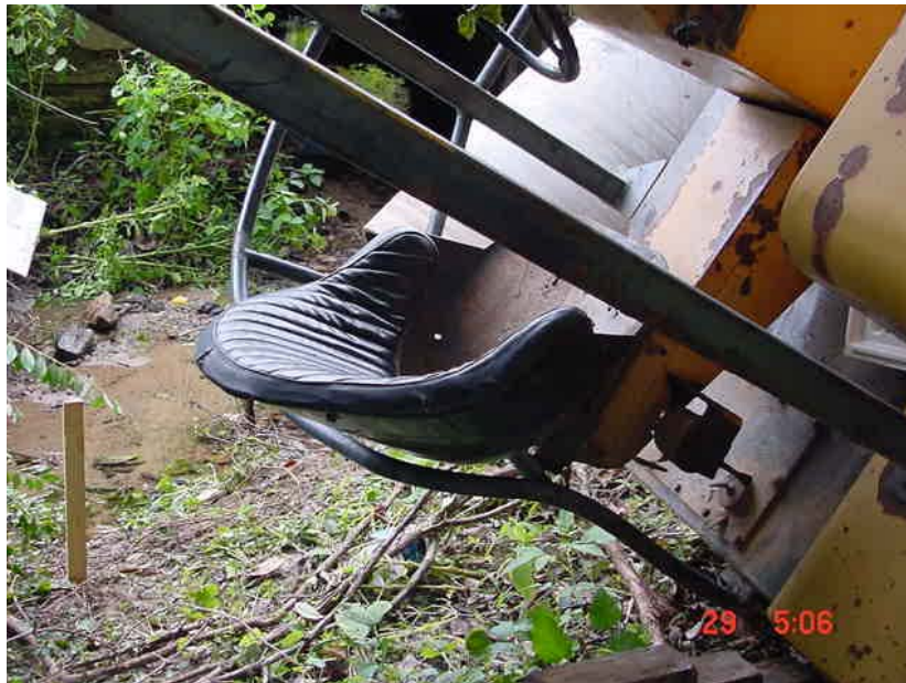
Figure 8. A seat and steering wheel perpendicular to the front of a compactor, which has no seatbelt; this unit was involved in an overturn-related death
