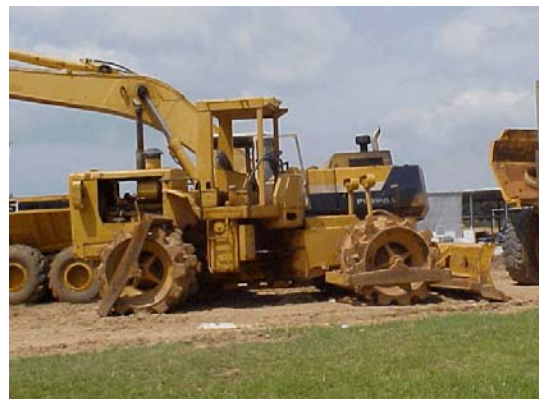
Figure 4. A double drum pad-foot compactor with articulated steering and a four-post ROPS with a canopy.
