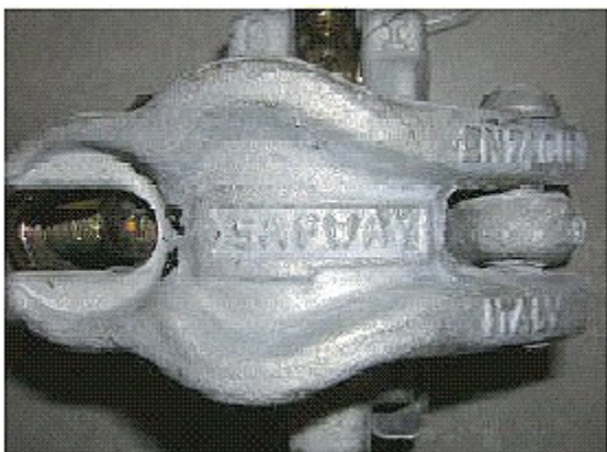
PHOTO 1 TOP SIDE OF A POTENTIALLY DEFECTIVE CAP SHOWING "SAFWAY" AND "ITALY"
