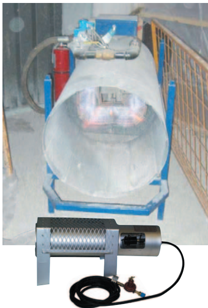
Salamander heaters mix fuel with air which burns in an open chamber.
