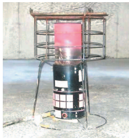
Infrared heaters work by burning fuel and heating an element until it glows red hot, thereby giving off radiant heat.
