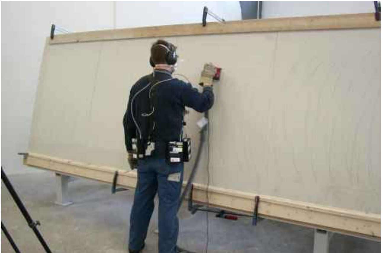
fig. 6.5.1 - 1 Test setup for orbital- and eccentric sanders
