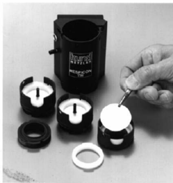
fig. 5.4.1 - 1 RESPICON and its three stepped collection system
