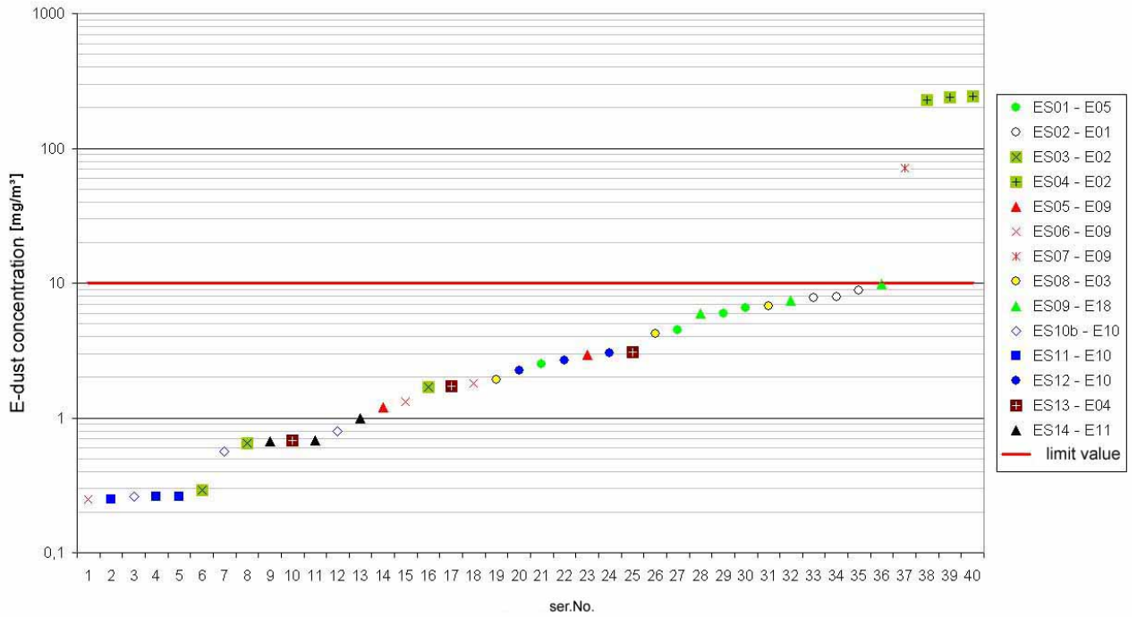
fig. 6.5.3 - 1 E-dust individual measured values for current eccentric grinders/sanders
