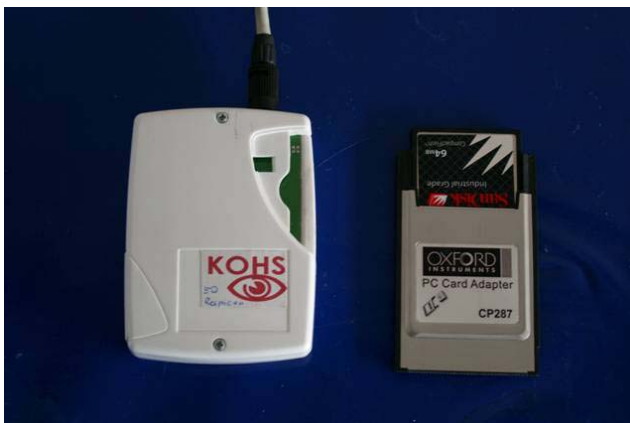
fig. 5.4.3 - 4 Bluetooth data logger and receiver on notebook
