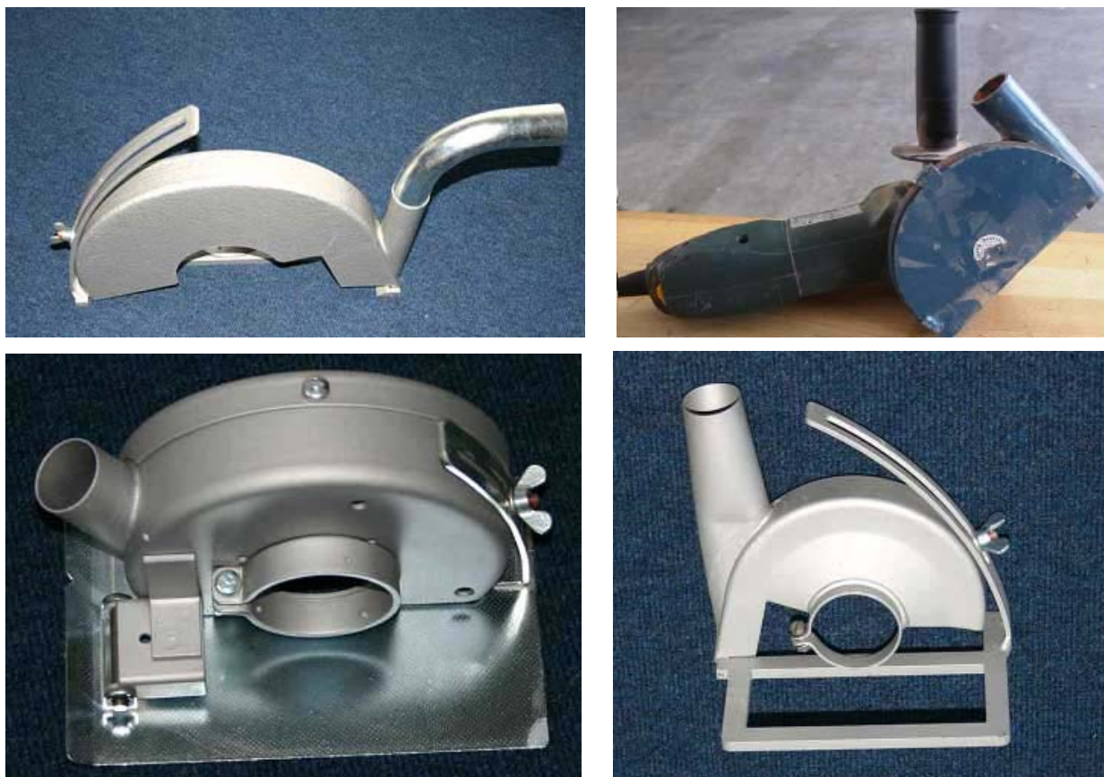
fig. 7.3.1 - 2 Examples of simple, stiff seizing hoods
