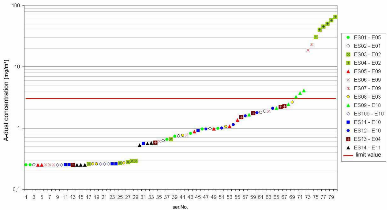
fig. 6.5.3 - 2 A-dust individual measured values for current eccentric grinders/sanders
