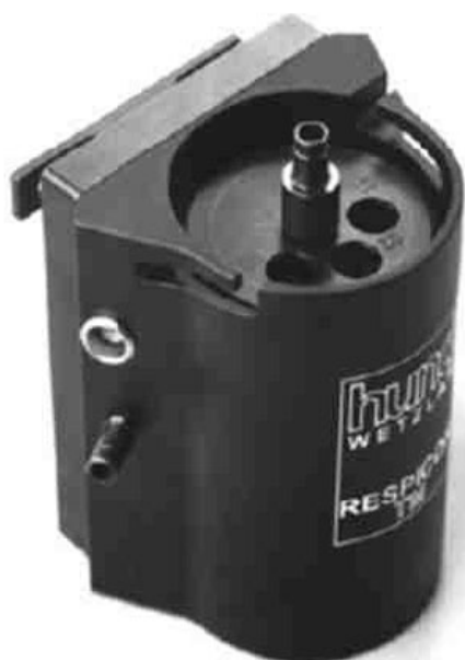
fig. 5.4.1 - 1 RESPICON and its three stepped collection system
