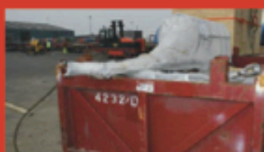
»» This unit is protruding both over the top and over the edge of the CCU causing a hazard to those involved in loading and offloading.
