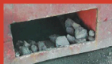
»» Loose debris in forklift pocket. This is a common occurrence which causes a hazard to road users and everyone involved in the lifting operation.
