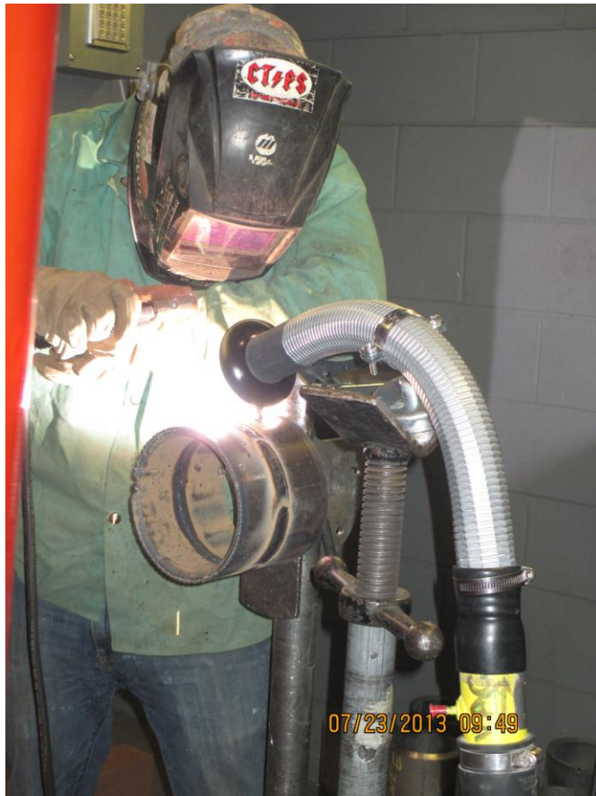
Figure 3: Welding carbon steel with LEV
