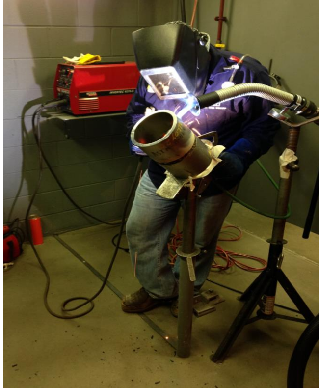
Figure 4: Welding Stainless Steel with LEV
