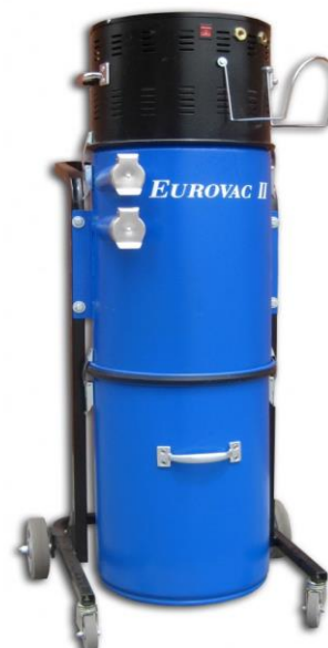
Figure 1: Eurovac II Welding LEV
