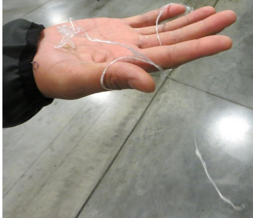
Example of a plastic “stringer” that would often tear off of the wrapping around the pallets of water bottles during loading and unloading and become caught on LGV forks. Stringers hanging from the forks that entered an LGV’s safety detection field would trigger an alarm and pause automatic movement.
