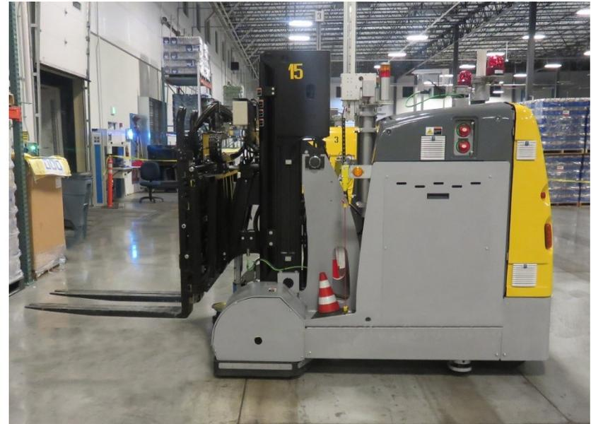
In December 2015, a 45-year-old warehouse dock coordinator at a water bottling company died after he was crushed when the elevated forks of an automatic laser guided vehicle came down on him.
